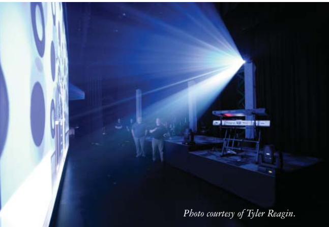
An ample backstage area houses Barco rear projection equipment that digitally delivers the video message onto the center screen. Barco's XLM HD30 30,000-lumen projector, and SLM R12 12,000-lumen projectors help make the magic happen.
